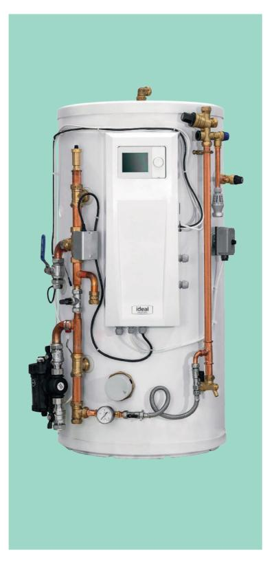
The two zone pre-plumbed cylinders include a lowloss header pre-plumbed onto the cylinder, decoupling the heating system from the heat pump, ensuring optimal flow and two zone control.
